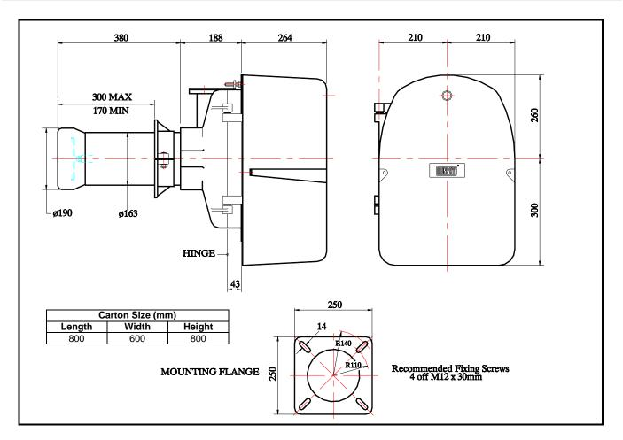
\*\* The burner gas train may be positioned as shown or rotated to the left or right as required.
