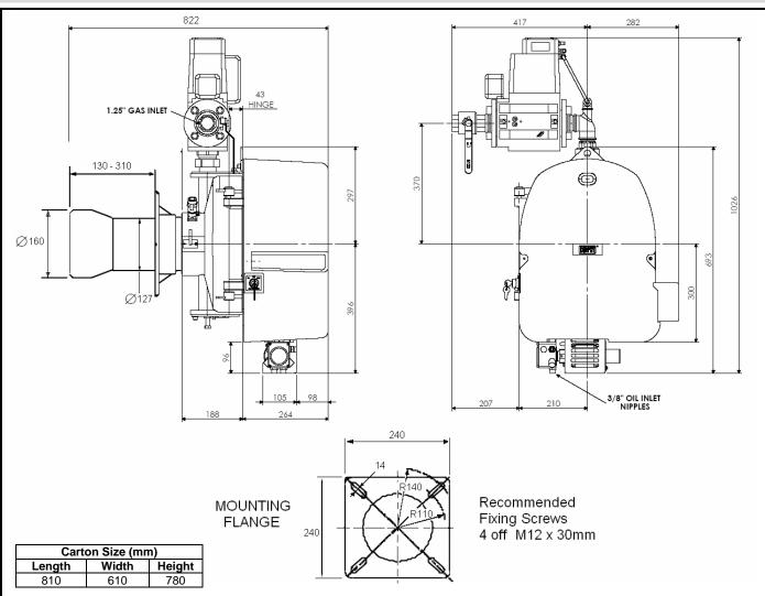
\*\* The burner gas train may be positioned as shown or rotated to the left or right as required.
